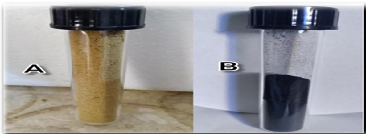
figure 8. [A] The date seeds and pomegranate peels powder after the carbonization process. [B] The activated charcoal. © Photography by the researcher.
