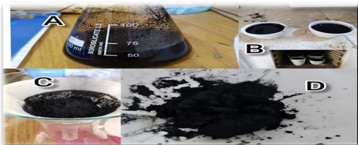
Figure 6. [A],[B],[C]and [D] show the steps of activation process by NaOH for the carbonated date seeds powder and pomegranate peels resulting from the carbonation process activated charcoal. © Photography by the researcher.
