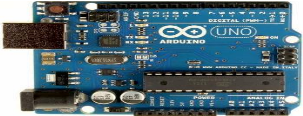
Figure 1: Arduino uno Open-source Microcontroller
